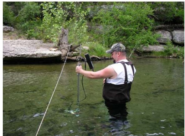
Eric Dedden using Flowtracker to measure streamflow in Cypress Creek, just downstream of Jacob's Well.
