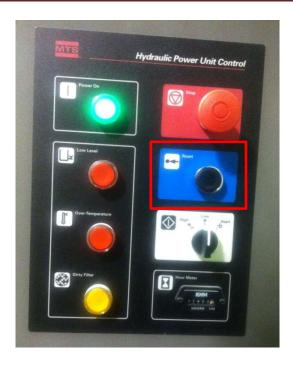
When you power up your controller, the hydraulic interlock will be set. Make sure to press the **Rest button** on the front of the Hydraulic Power Unit Control or interlock will be set.
