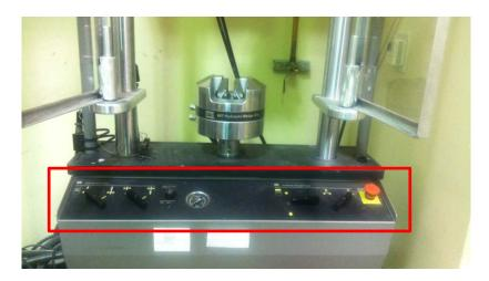
Make sure that the upper and lower grip control knobs are in the decompressed state. Make sure that the upper crosshead control knob is in the compressed state. Make sure that the Emergency Knob is not pressed in.
