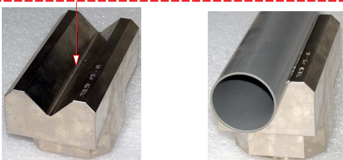
Fig. 2 - Pipe Support 90° code 7520.210 according to ASTM D-2444 standard for pipes diameter 25 to 65 mm (to be used together with the adjustable height support code 7520.035)
