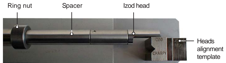
Fig. 9 - Striker with the Izod head aligned
