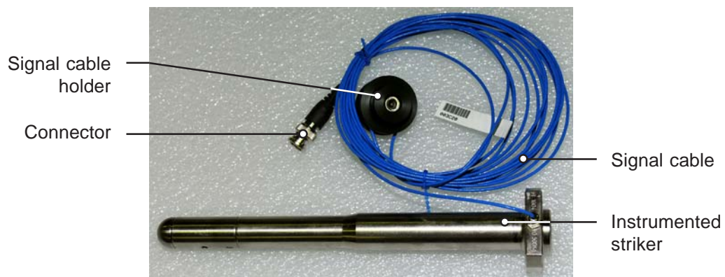
Fig. 1 - Instrumented striker (usable with both striker holder)
