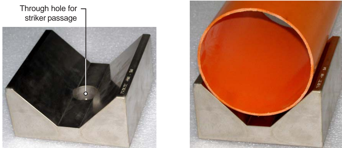
Fig. 1 - Pipe Support 90° code 7520.212 according to ASTM D-2444 standard for pipes diameter 80 to 160 mm (to be used together with the adjustable height support code 7520.035)
