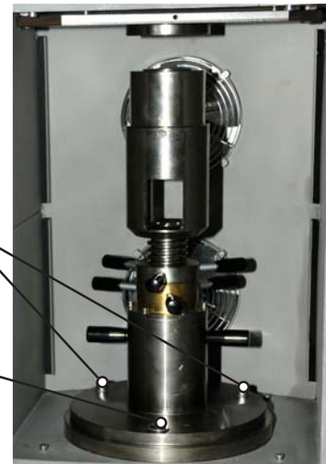
Fig. 2 - Adjustable height stand
