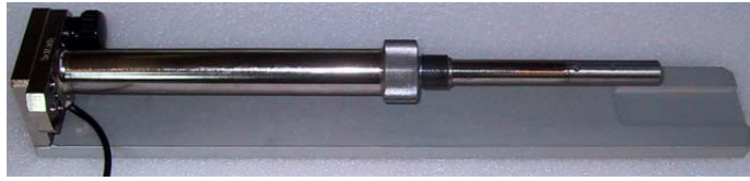
Fig. 7 - Striker body fastened to the fixture without head and spacer
