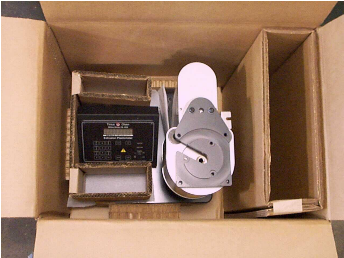
Figure 23-3 (This picture shows the Melt Indexer securely in place with the foam on the table under the cardboard divider.)
