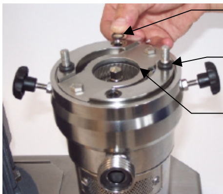
Place premounted stator unit
