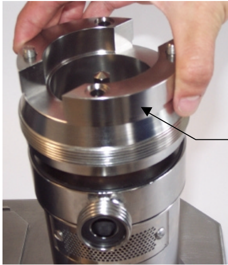
Premount stator with adjusting ring
