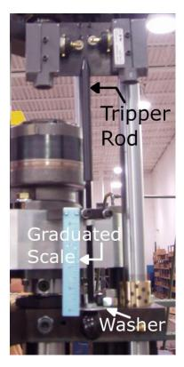
the 3" mark. There is a loss of about 10% of the shot size due to material lost in operating the sliding non-return valve in the screw tip, so that must be taken into account.
