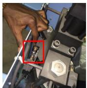
17. Set the cycle and injection timers to the values observed during your manual set-up. Injection time should be sufficient to have the screw motion stop. If your cavities are of thick section, both longer injection dwell and overall cycle time should be lengthened to prevent "sinking" of the part.
