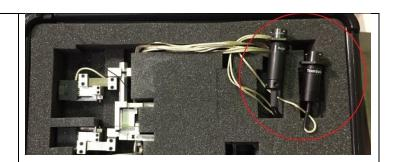
Connect the two cords of the Biaxial Extensometer called "Transverse" and "Axial" to the cords available on the left of the MTS machine called "Transverse Disp gauge" and "Poissons Axial" resp.
