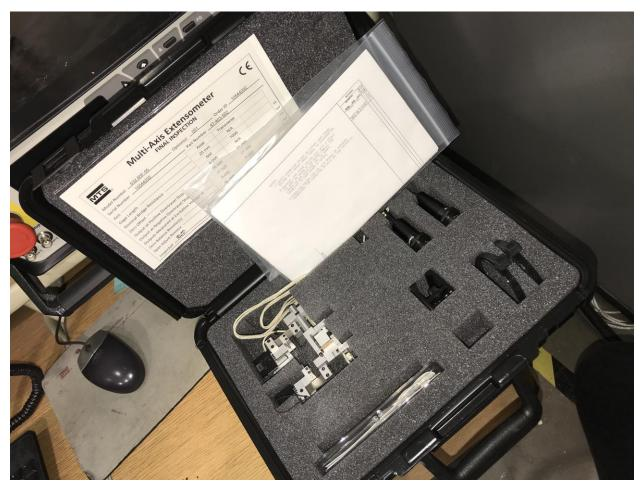
Biaxial Extensometer located in table cabinet labeled "MTS GRIPS, EXTENSOMETER"
