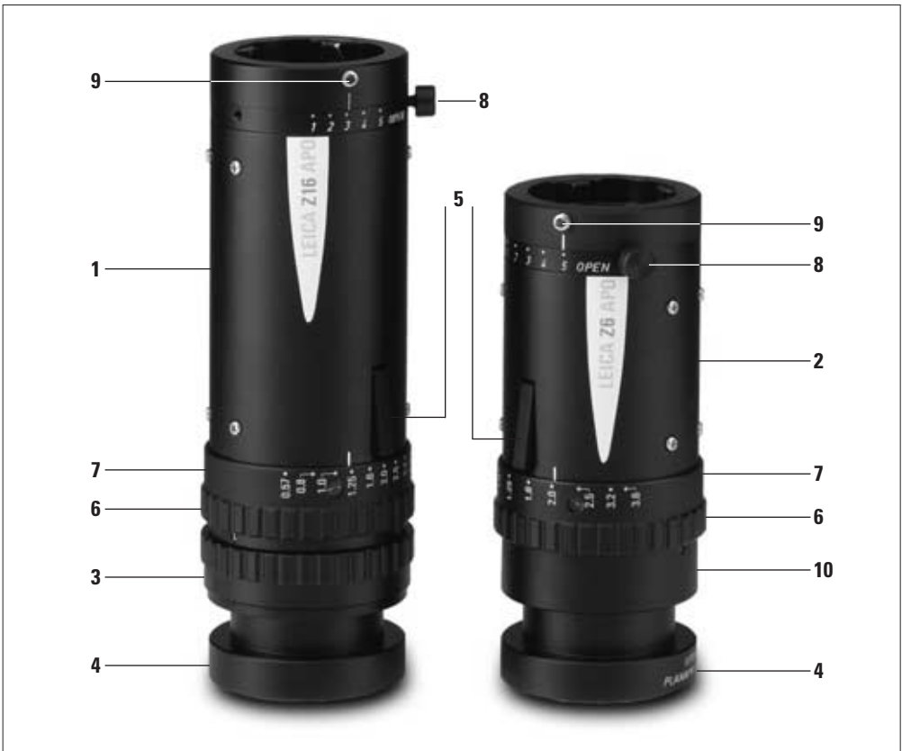
Fig. 1 Basic components and controls: left, Leica Z16 APO zoom system with fine focusing and objective. Right, Leica Z6 APO zoom system with objective.
