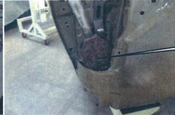
Add an enclosure to coil spring to reduce zinc shot debris
