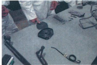
Add an enclosure to coil spring to reduce zinc shot debris
