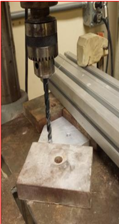
Drill press to create holes in the gusset plates
