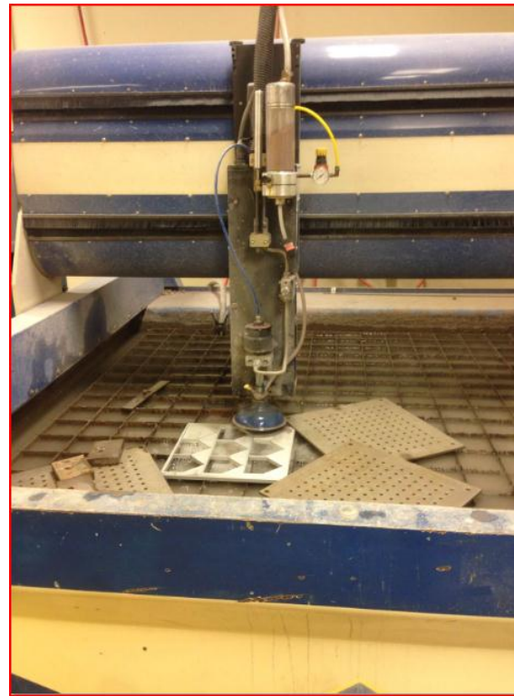
Water jet to cut gusset plates
