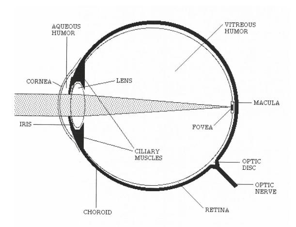
NOTE: The diagram shows a laser beam entering the eye and being focused on the fovea. If the beam power is sufficient, this situation could cause blindness.
