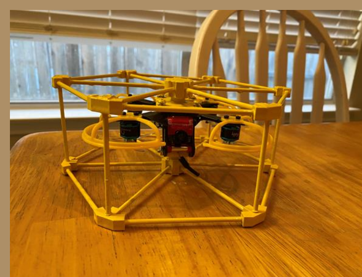
Drone Cage Assembly
