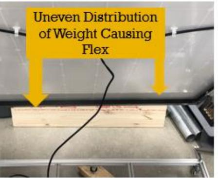
The proposed idea was to find a way to distribute the weight of the solar panel evenly. Centering the actuator in the middle of the
