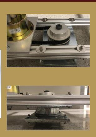
$\succ$  These different designs were made to constrain the pully to the shoulder screw and then have it fixed to the bottom plate of the
