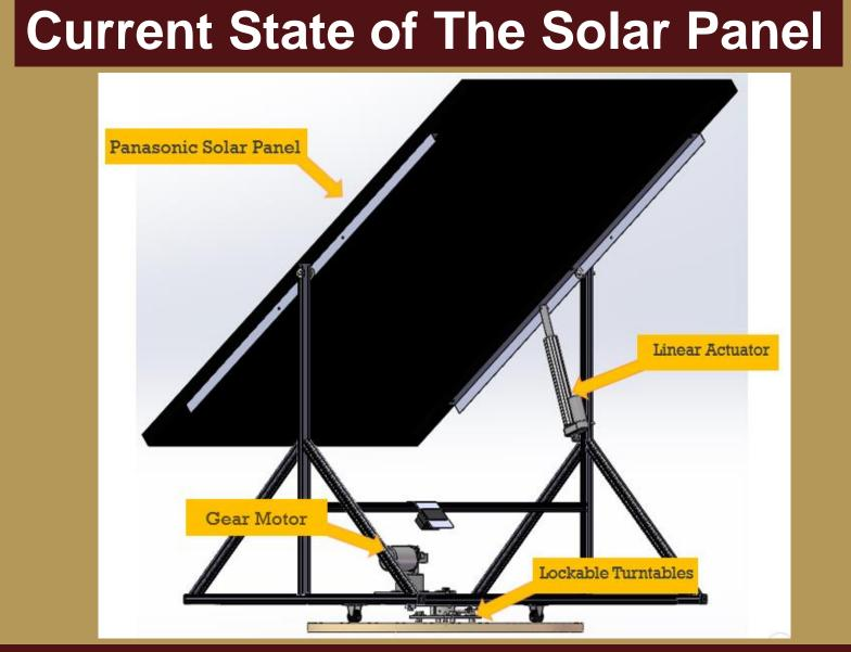
> The overall goal of this project is to get the solar panel to orient itself to face the sun with the use of a GPS tracking system. > With that major goal in mind, our customer has presented our team with few problems that focus on the azimuth mobility of the solar panel.
