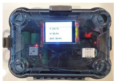
Our product is a lightweight and low-cost heat island mapping device designed to collect, record, transmit, and use data to create a color-coded virtual map. The device can collect up to 5-hrs of data at a time, store at least one month of daily recorded data, and transmit the recorded data to cloud storage via Wi-Fi.
