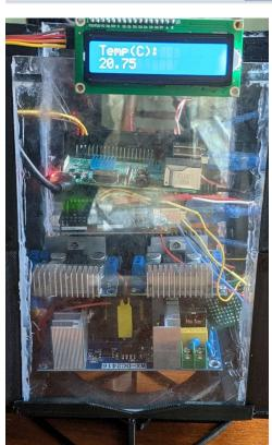
Smart Leaf combines technology and gardening to create a new method for growing food. Our system can detect and alert the gardener to any unwanted growing conditions that the plant may be in. The system will also store this data for the user to analyze and determine trends in the environment. It does all of this while fitting into a ergonomic water-resistant case affixed with RGB lights that indicate the status of the system.
