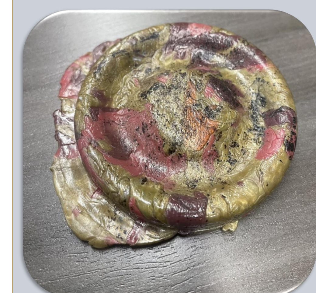
Carbon build up
