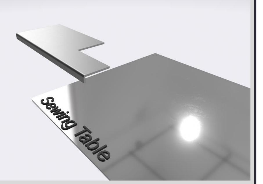
This right-angle tool lies flush on the bottom left corner or the operator's workstation. Edges are bent to catch on the edge of the table
