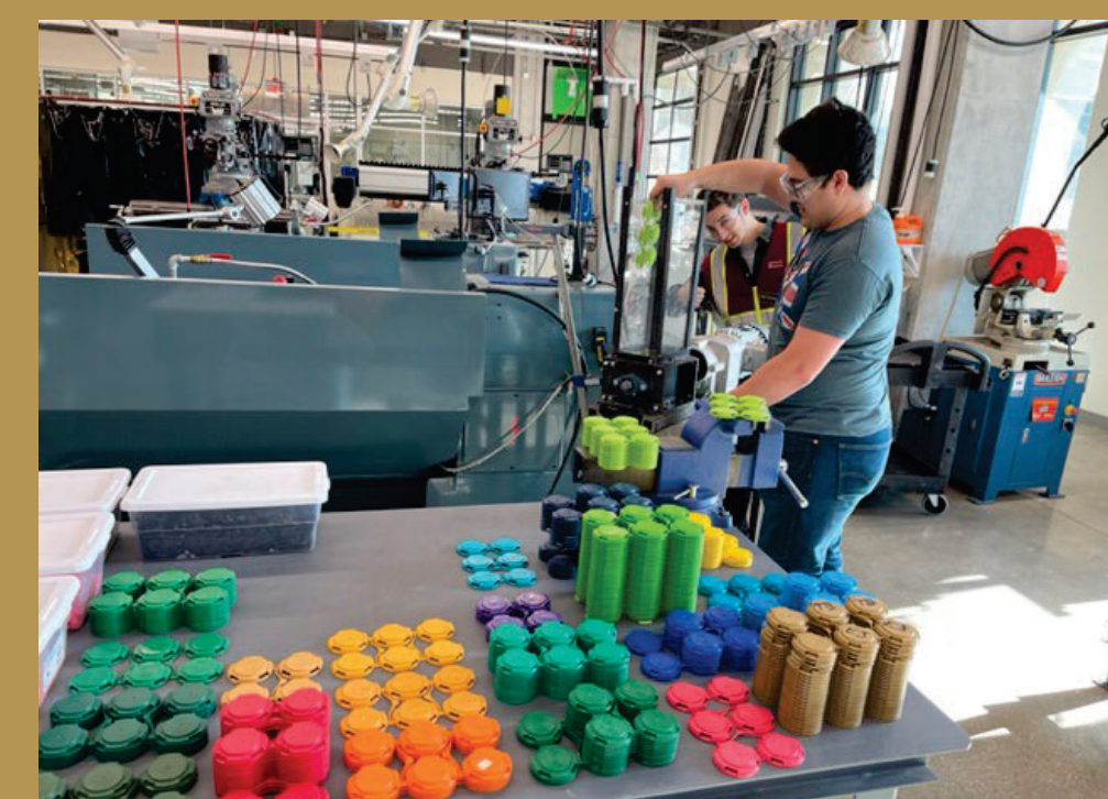
Figure 1: Shredding HDPE plastic
