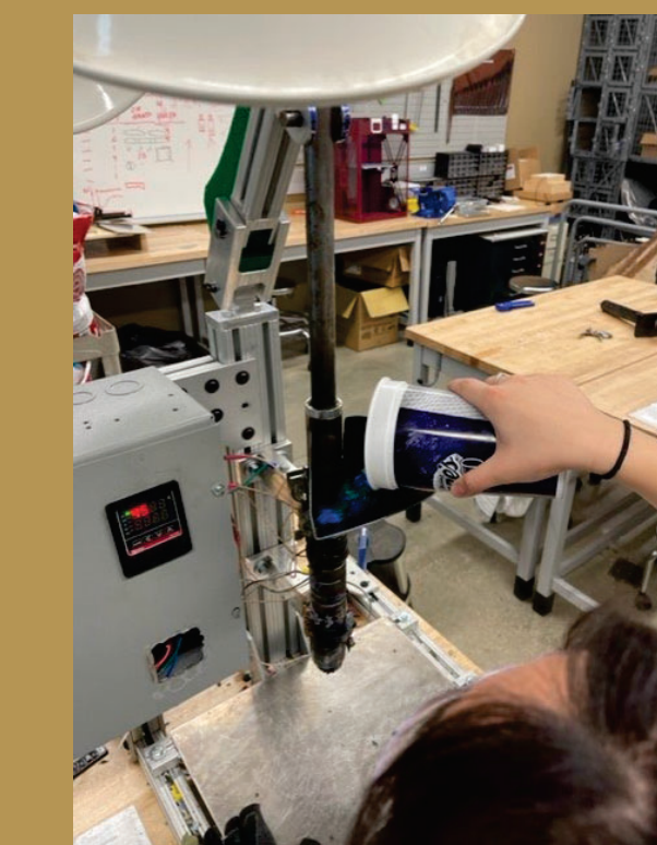
Figure 11: Loading of the plastic into the barrel
