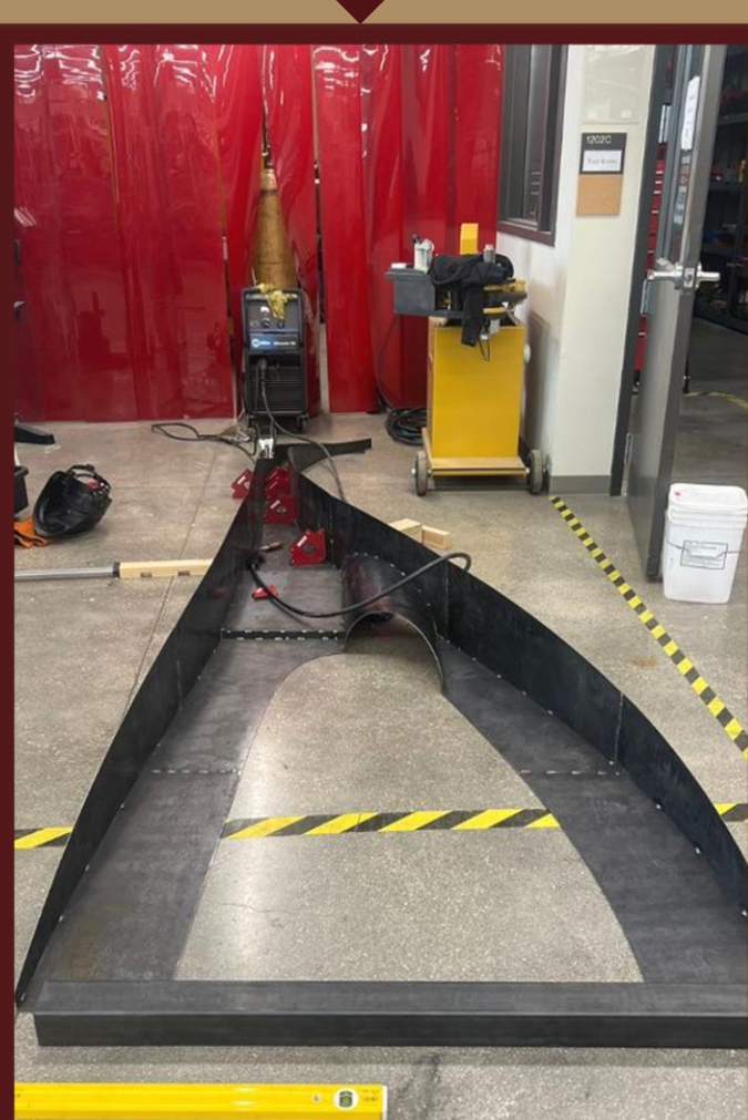
Rolled 6" Radial Tunnel
