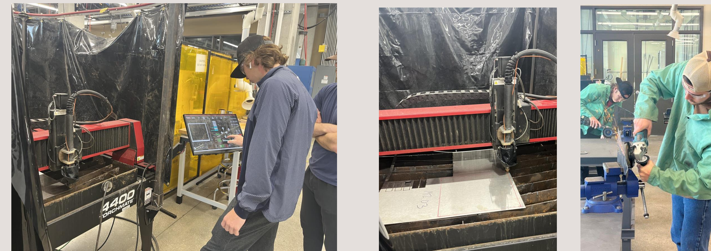
Plasma cutting the pieces for the hopper
