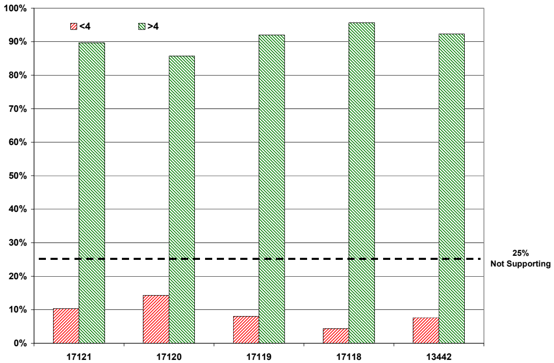
Fig. 17. Percentages that 24-hour mean DO concentrations exceed a 4.0 mg l -1 criterion for all values recorded from August 2000 through October 2001.
