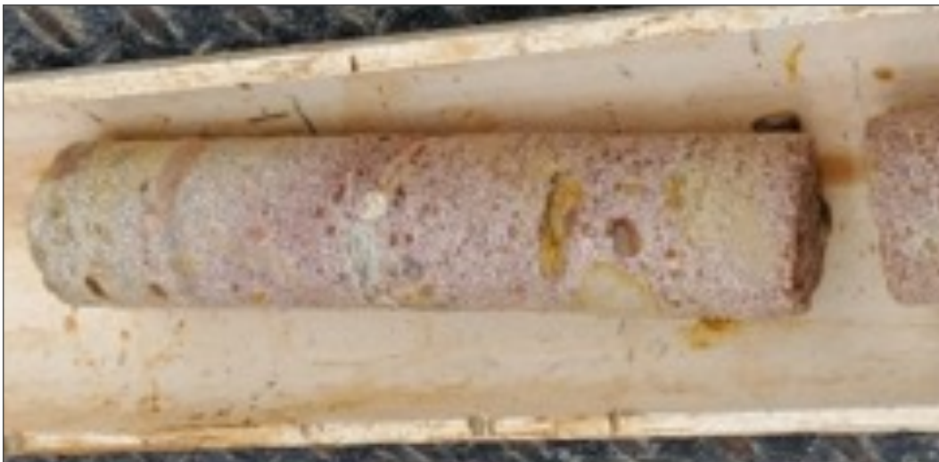
FIGURE 6. CORE SAMPLE OF THE SYCAMORE CONGLOMERATE AT MW4
