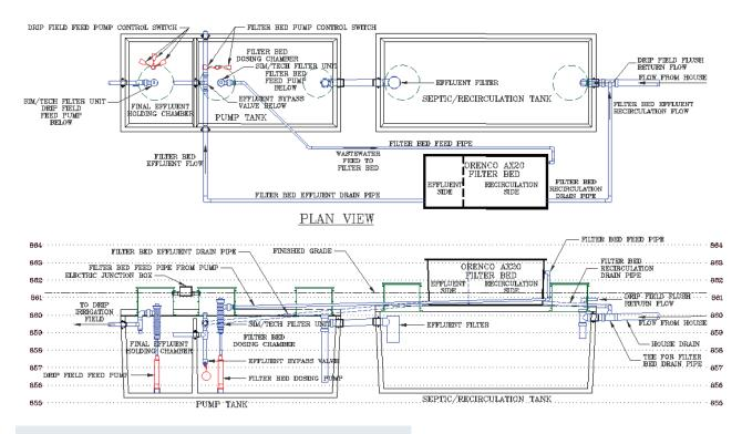
Figure 8. Recirculating Packed-Bed Filter Treatment Unit
