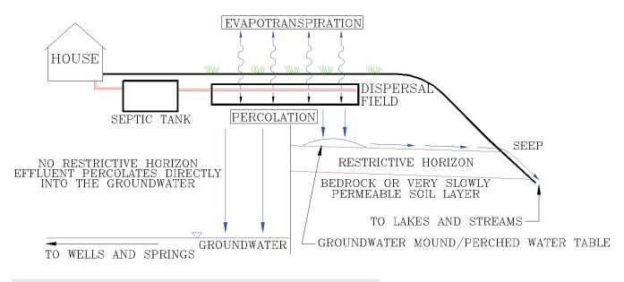
Figure 3. Fate of Wastewater Discharged to OSSF Dispersal Field
