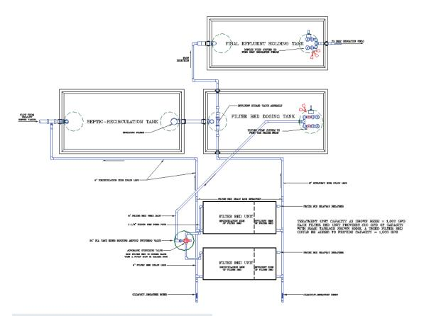
Figure 10. Collective System Treatment Unit
