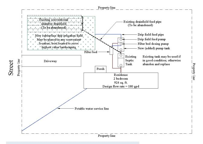
Figure 9. Recirculating Packed-Bed Filter–Drip Irrigation OSSF Retrofit
