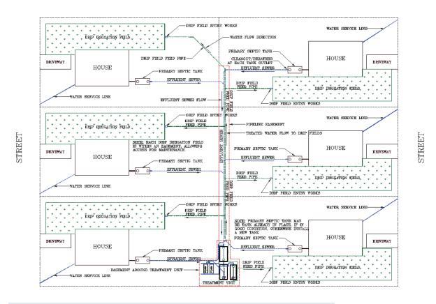
Figure 11. Small-Scale Collective Collection, Treatment & Dispersal System
