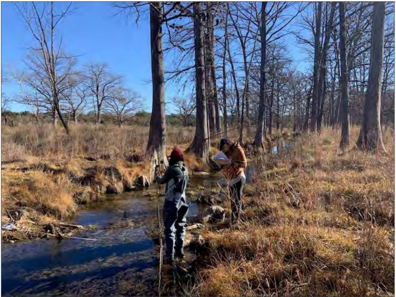
Figure 5. Meadows Center staff measuring flow with the Sontek FlowTracker sonde
