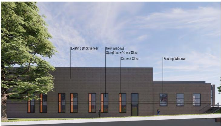
North Elevation - Existing Building with new windows
