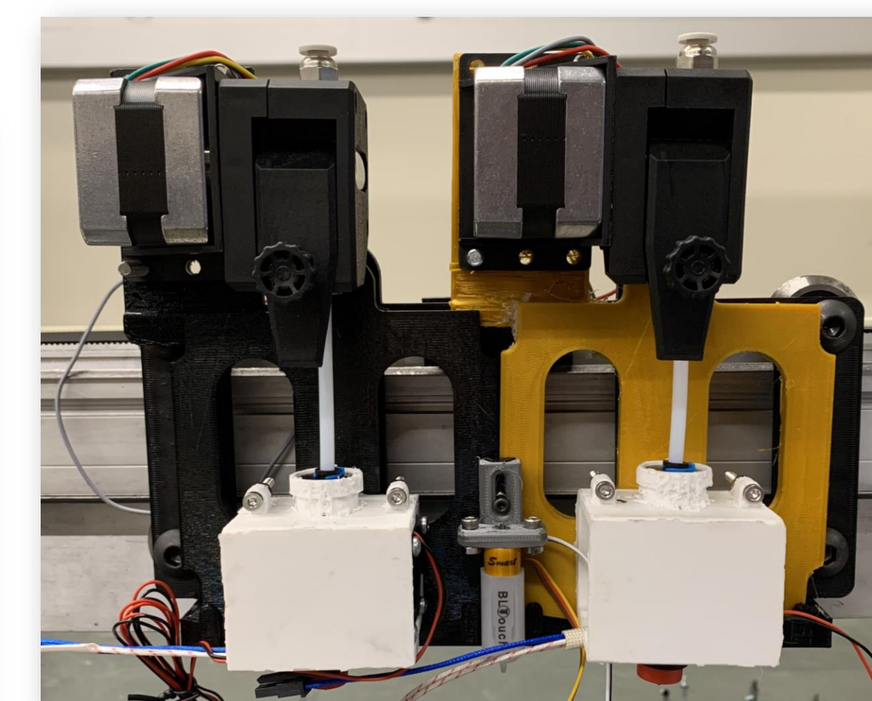
Former extruder set up (left) and the redesigned extruder mounting system (right)
