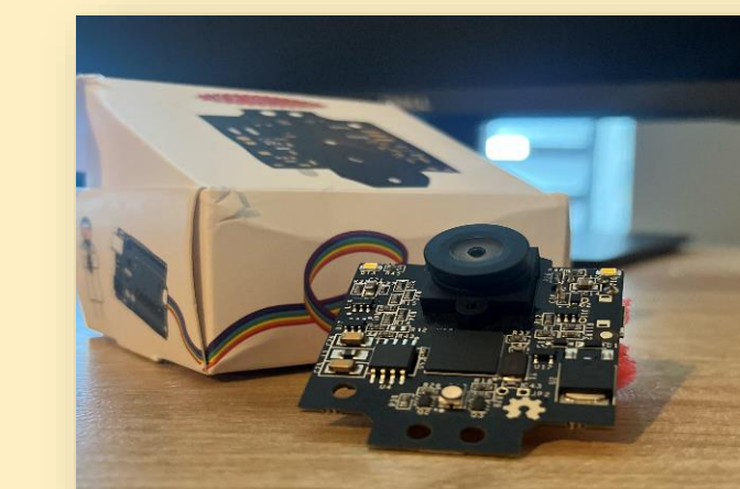
Pixy 2.1 CMUcam5 Image Sensor
