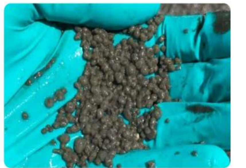
Granule sample following sieve testing at the AquaNereda ® demonstration facility, Rockford, IL
