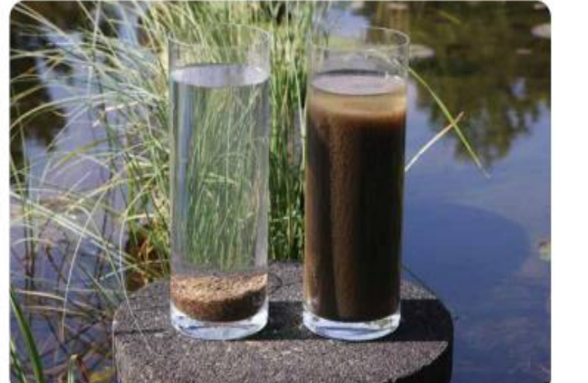
SVI comparison of aerobic granular sludge (left) and conventional activated sludge (right)
