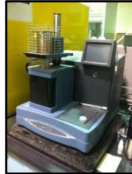
TMA Q400 Temp. Range: -150C to 1000C Force Range: 0.001 to 2N
