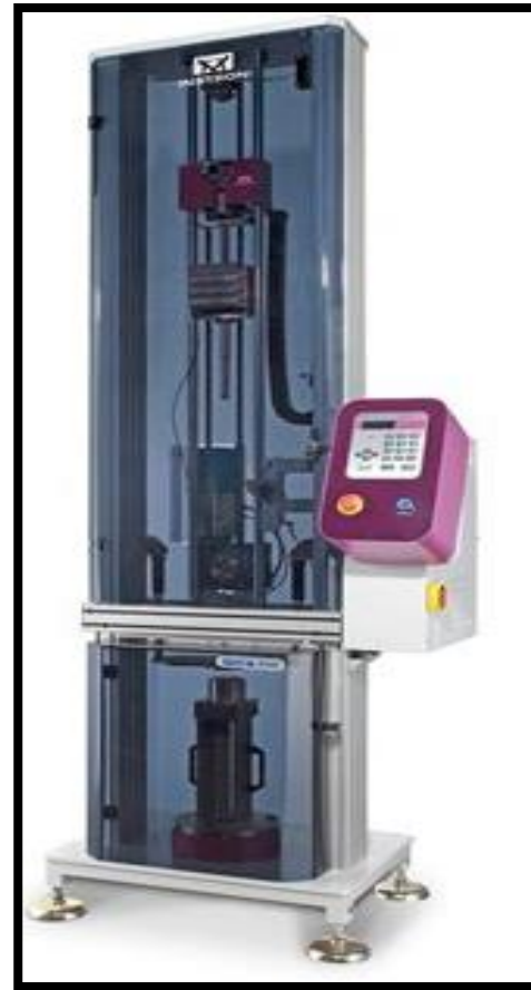
LOW VELOCITY DROP TOWER IMPACT TESTER Max. Energy: 405J
