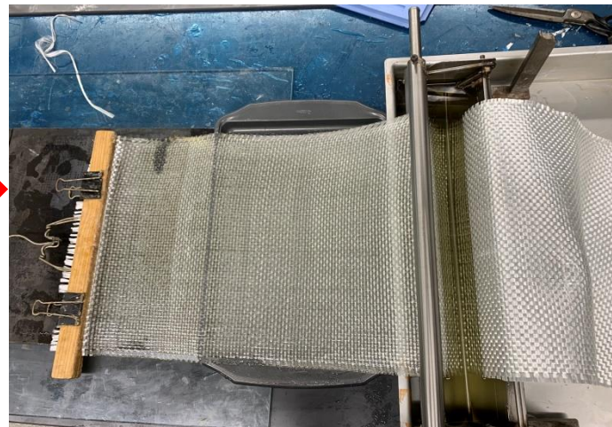
E-Glass fabric being pulled through the resin bath
