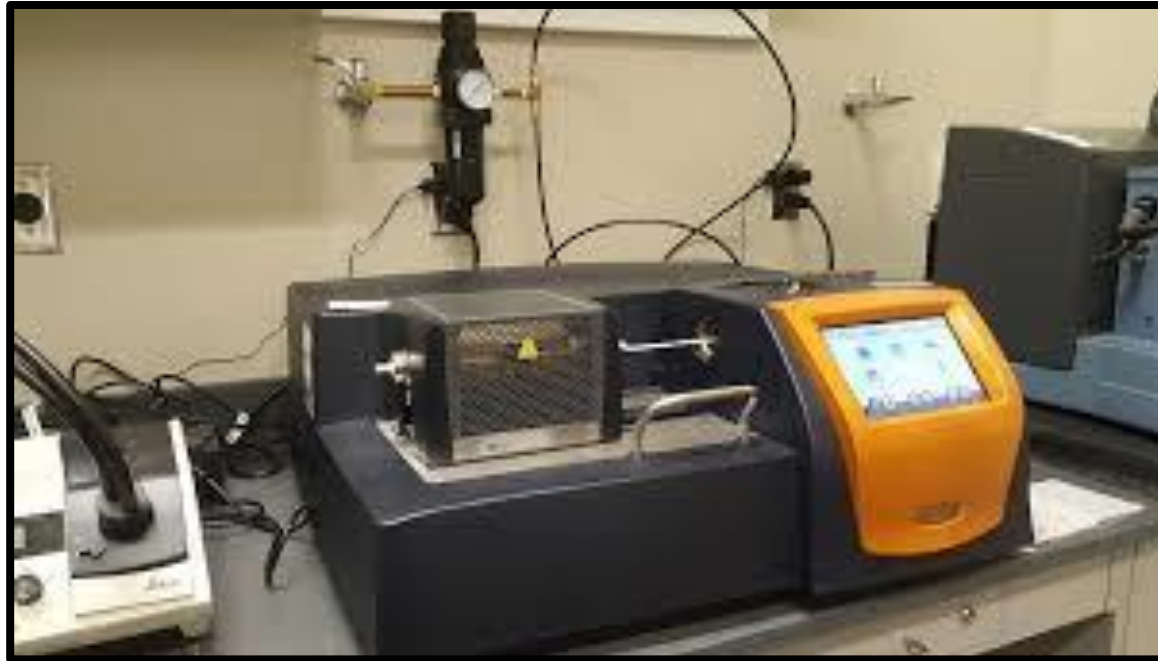
DISCOVERY 650 SIMULTANEOUS DSC TGA Max. Temperature: 1500 C
