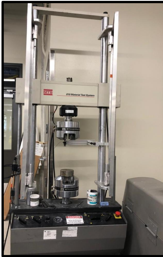
MTS SERVO HYDRAULIC TESTING EQUIPMENT Max Load: 100kN
