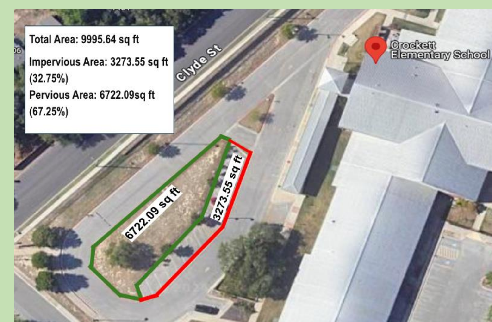
Figure 3: Biogarden Drainage Area Consideration
