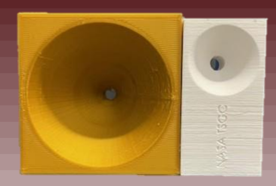
Fig. 2: The size reduction between the first conical horn (left) and the final horn design (right).
