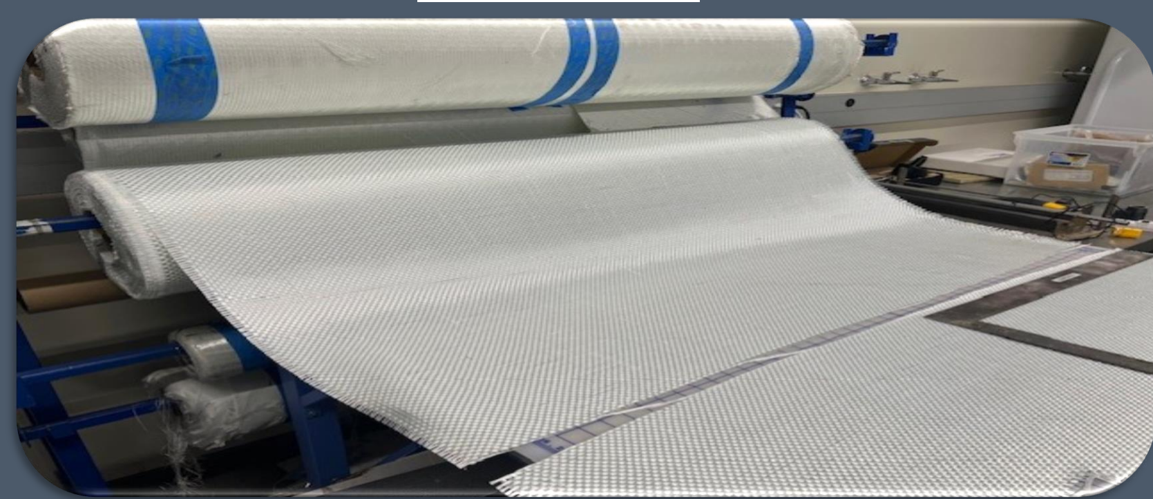
E-Glass Fiber Weave Pattern: +/- 45 degrees stitched
