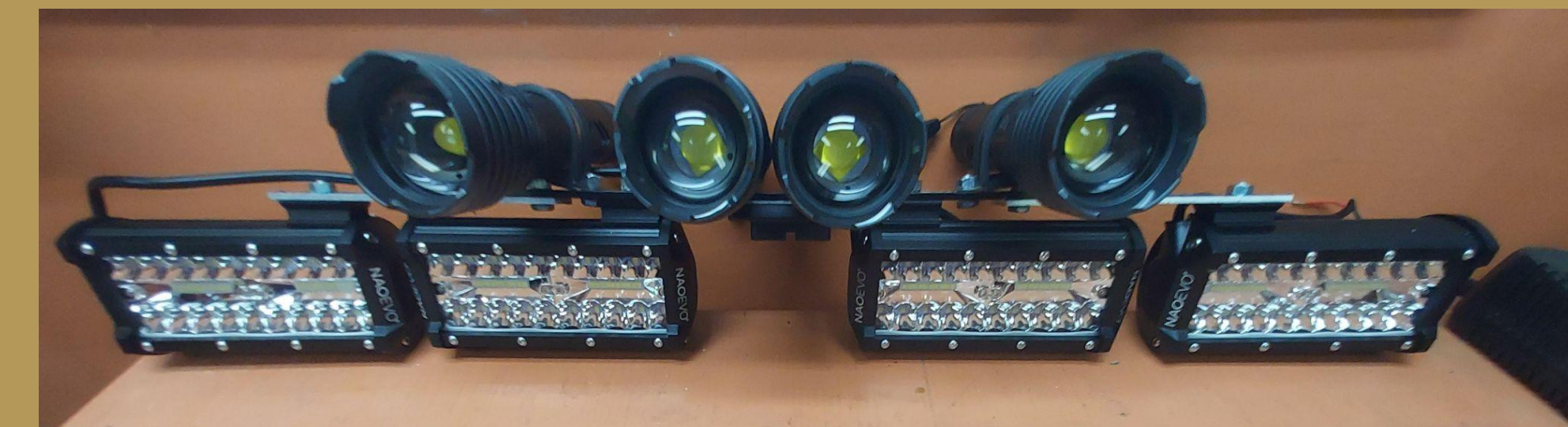
The lighting array is made up of four independently dimmable spotlights and two banks of floodlights, all driven by the image processing scene data.
