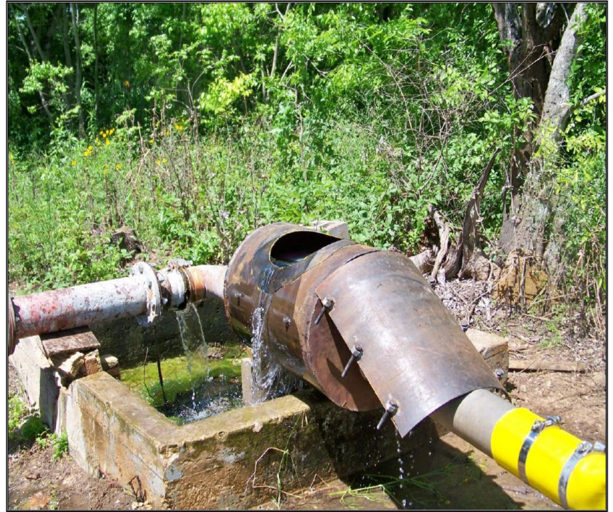
In line barrel sampler on an irrigation well in Bexar County, Texas.
