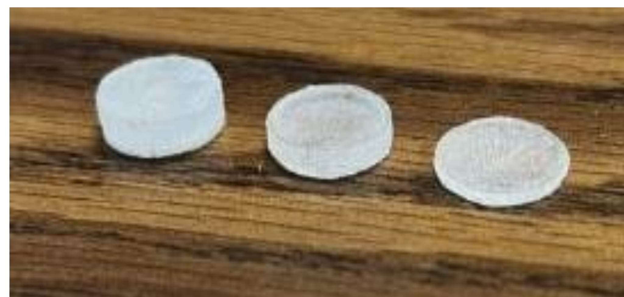
Mark1 - 3D printed sound dampening buffers, each a different thickness to test its effectiveness
