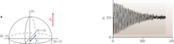
Fig 5: A: The Bloch sphere. A point on the surface of the sphere describes a possible qubit state. C: Rabi oscillations of switching probability..
