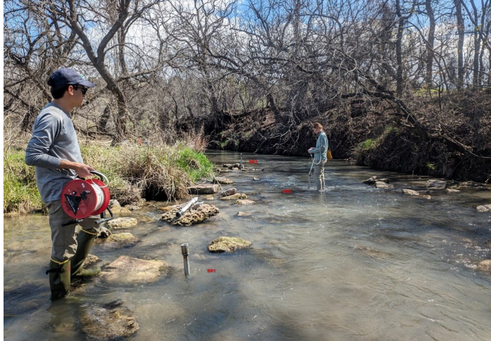
Taylor McNair collects water from the hyporheic zone in the Pedernales River, while Joseph Aubert prepares to get water-level measurements.
