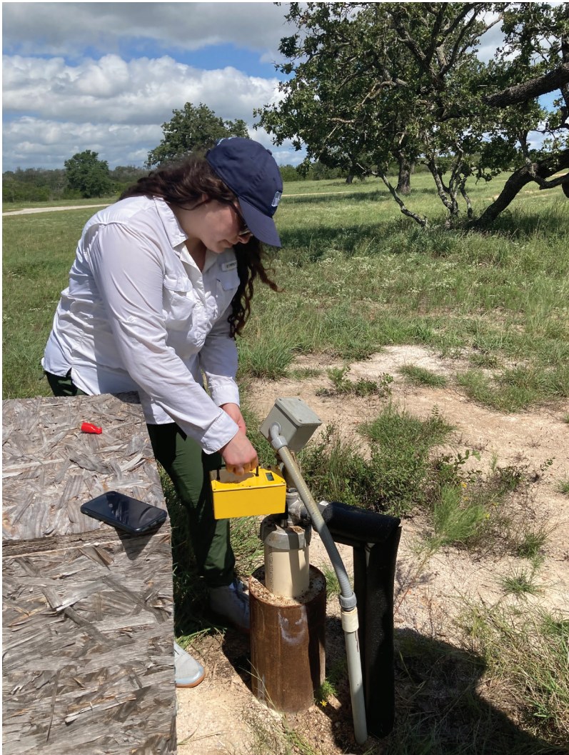
Figure 11. MCWE staff conducting a well level measurement using a sonic meter (photo credits: Nicky Vermeersch)
