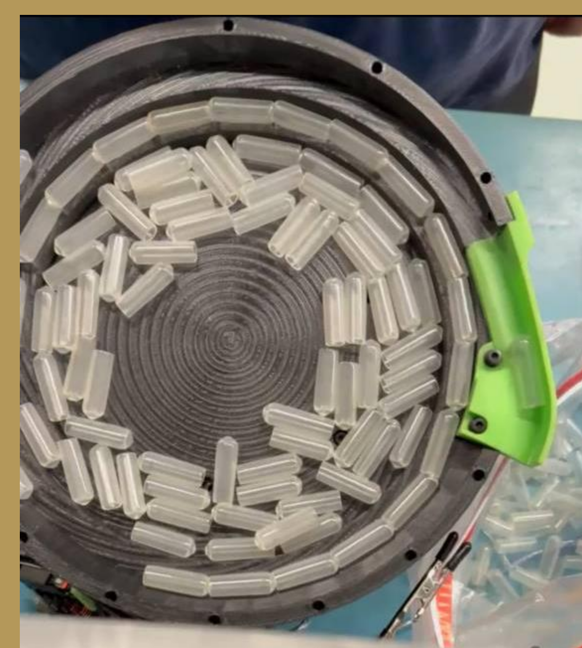
Left: Auxiliary Views of Bucket Hopper Right: Physical Model of Vibratory Bowl Feeder, also shows EZ pen cap part.
