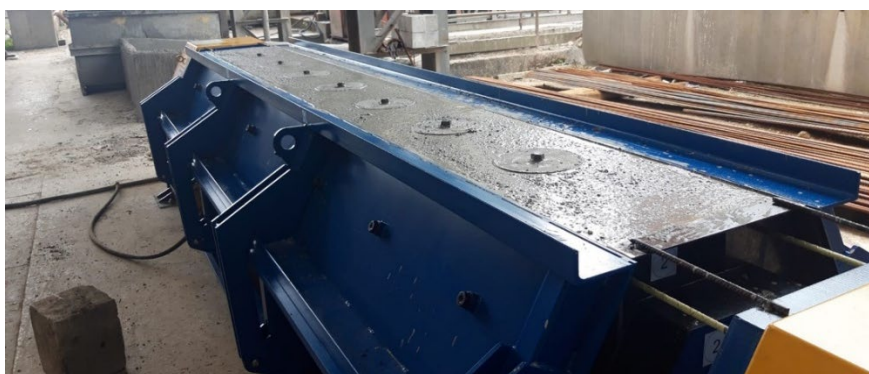
Figure 6: Final prestressed GFRP SEAHIVE® module in the conical steel mold after concrete casting (Patent pending filed by SIGMAc s.r.l., Vicenza, Italy).
