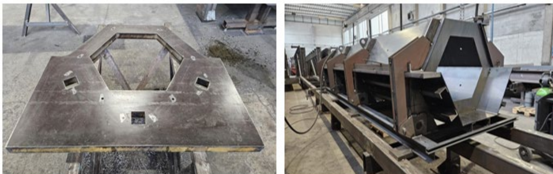
Figure 3: Fabrication of steel molds for SEAHIVE® modules (Patent pending filed by SIGMAc s.r.l., Vicenza, Italy).
