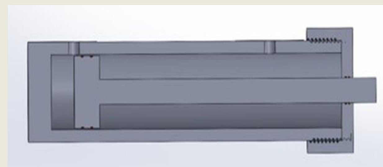
Double Acting Roll Cylinder Cross-Section
