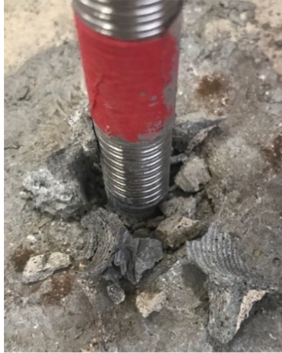
Figure 24. TiAB pullout failure at concrete-ECSG interface (note how TiAB deformation surface is visible in ECSG).
