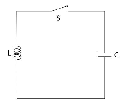
The induced voltage across the inductor must be equal to the voltage across the capacitor. The sign of this equation however depends on the direction of the current. If the current flows towards the positive plate of the capacitor the sign should be negative, if the current flows away from the positive plate of the capacitor the sign is positive.
