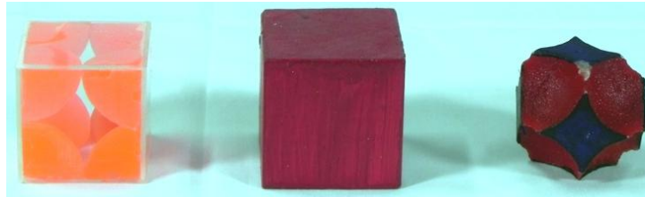
Fig 2: central void in center of simple cubic crystal structure.
