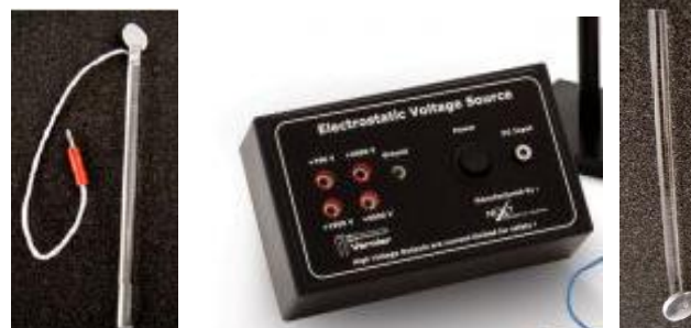
Fig. 3: Voltage terminal, Electrostatic Voltage source, and proof plane
